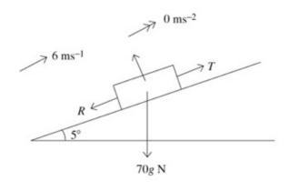
Power =  $F \times v$   $480 = T \times 6$   $T = \frac{480}{6} = 80$   $R(\rightarrow)T = R + 70g \sin 5^{\circ}$   $80 = R + 70 \times 9.8 \sin 5^{\circ}$   $R = 80 - 70 \times 9.8 \sin 5^{\circ}$  R = 20.21The magnitude of the resistance is 20.2N.
